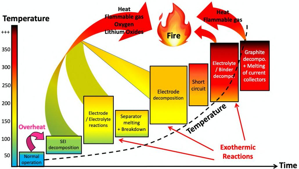
**Runaway** happens when additional **overheat** cannot be dissipated fast enough
